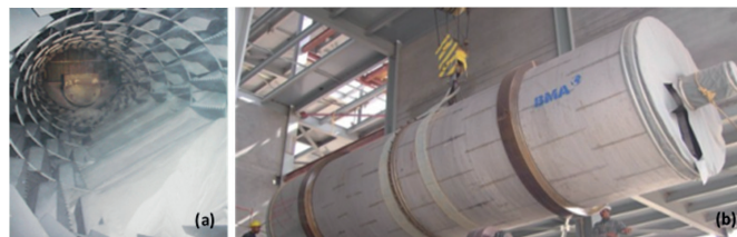
Figure 6: (a) Drum dryer in stainless steel; (b) drum with riding rings in mild steel
