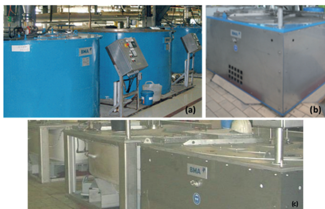
Figure 5: (a) Old continuous centrifugal with mild steel housing; (b) continuous centrifugal K3300 with stainless-steel housing; (c) continuous centrifugal K3300 with complete stainless-steel housing
