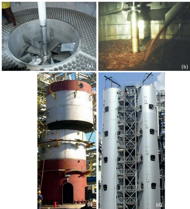
Figure 3: Vertical continuous pan VKT: (a) calandria in solid stainless steel; (b) vapour chamber clad in stainless steel; (c) VKT during assembly; (d) VKT insulated
